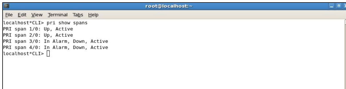
A screenshot of a terminal window titled "root@localhost:~". The window shows the command "pri show spans" being run and its output. The output indicates four PRI spans: span 1/0 is Up and Active; span 2/0 is Up and Active; span 3/0 is In Alarm, Down, and Active; and span 4/0 is In Alarm, Down, and Active.
